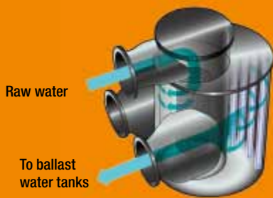
Figure 1 – During ballast water intake, water passes through both the filter and UV disinfection.
